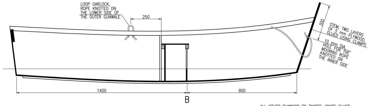
ALL OTHER PLYWOOD TO TIMBER JOINTS GLUED AND NAILED WITH 1.2 x 20 mm NAILS SPACED 50 mm
